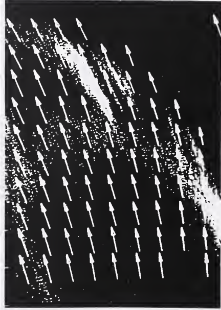
Figure 4 A sample double image of smoke seeds flowing into a fire obtained with the Particle Imaging Velocimetry (PIV) instrument.
